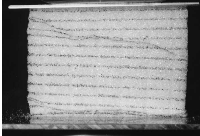
Fig. 6. Two deformation bands within a specimen.
